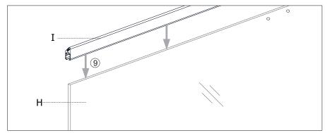
▲ Check the aluminum alloy door magnetic strip if installed well; Make sure it and then install the hinge on the open door.
