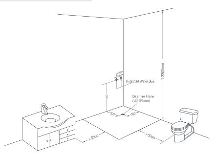
2.1) Drainer: try to make the drainer on top of the water outlet position; if it isn't possible to make sure, it should be set up at least 300mm in the water outlet, the diameter of water outlet should be less than 500mm.
