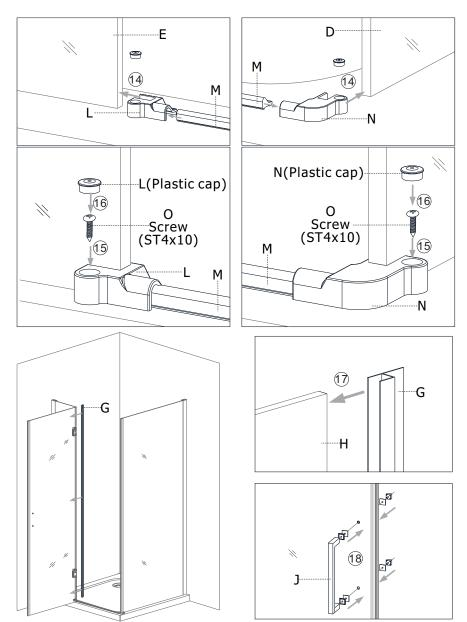
4.1) Two persons will be better for installation , please take up the open door ,and insert the hinge onto the fixed glass ,put well the gasket ,and then fasten the hinge by its screws ;Adjust well the location of aluminum door magentic strip between open door and lateral door ,make sure it will be good .
