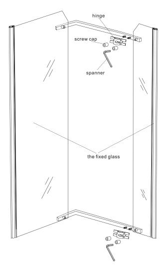
6.1) fix hinge into glass by spanner.
