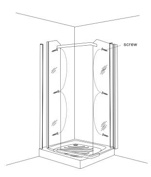
5.2) Put the bracket on the shower tray and use the screw fix the bracket in the side glass
