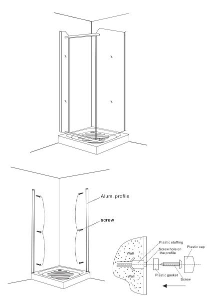
$5.1)\mbox{Put}$  the frames on the shower tray , draw the frame place, then take out the sild profile and fixed it.
