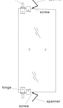
6.2) fix hinge into glass by spanner.
