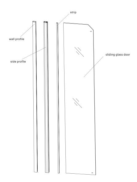
4.1) assemble wall profile, side profile, strip, side glass together.
