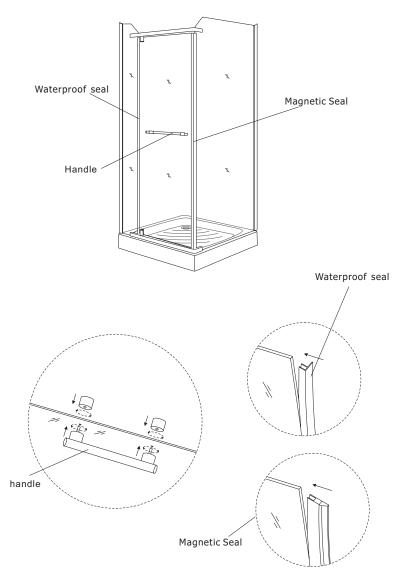
Assemble the door handles, waterproof seals and the magnetic seals with the glass door respectively. (as per the above drawings)
